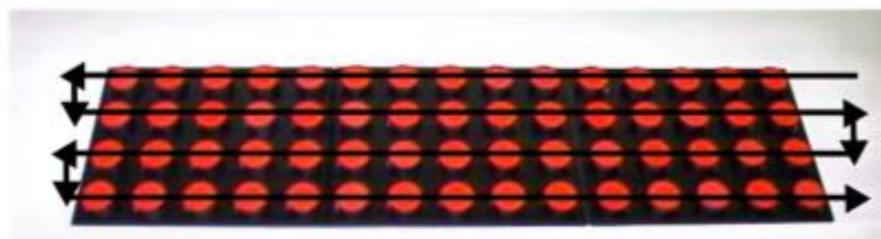
Figure 4: Starting position and sequence of rows with directions of travel for the Turning Test.
